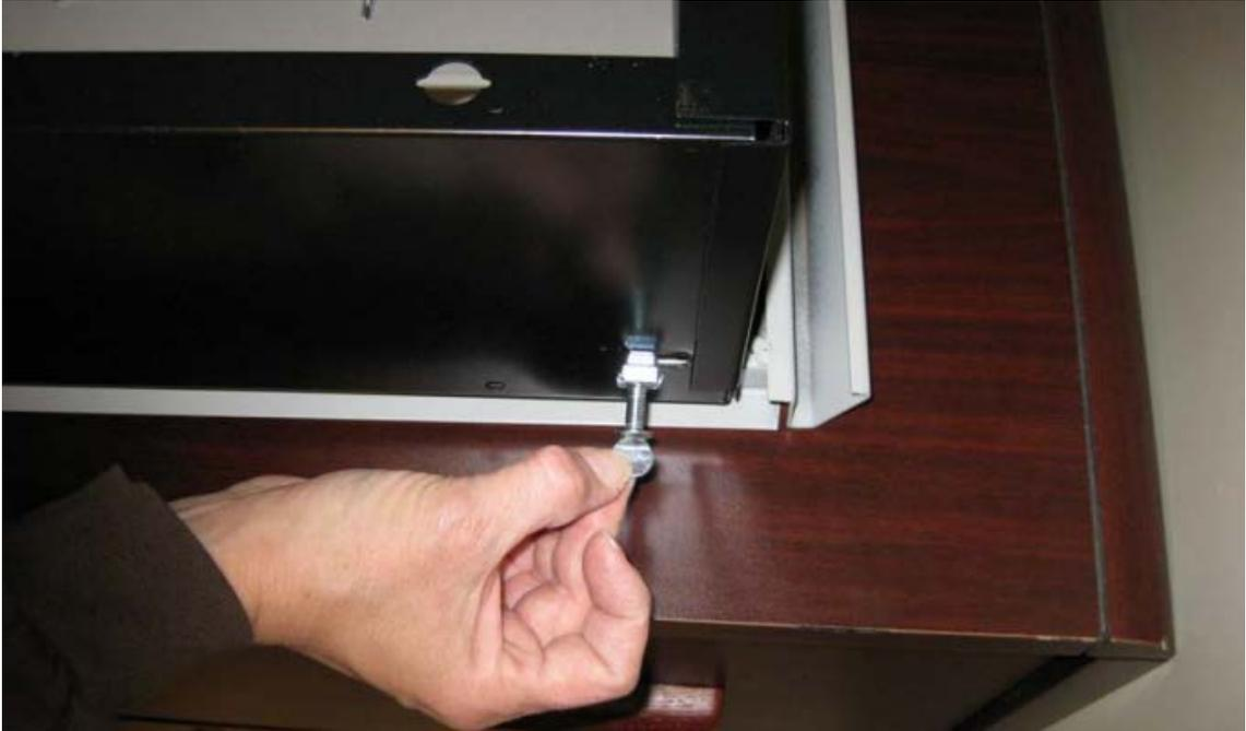
Insert from thumb screw into openings on either side of the back. Remove thumb screw and put through opening on the gondola and screw in tight to attach.
