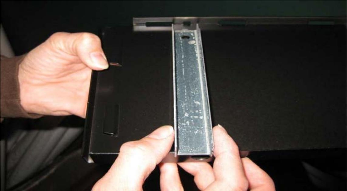
Insert tab on bar into the small hole on the lip.
