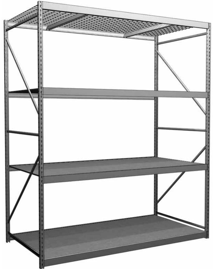
**WARNING:** Multi-Function Beams are intended to be used with Multi-Function Shelf Supports. If Shelf Supports are not installed then the beams MUST utilize a Widespan Multi-Function Beam Locking Clip (WS1291 or WS9111 pg.706) depending on the beam location. Failure to do this could allow the Beam to become disengaged causing product damage or personal injury.
