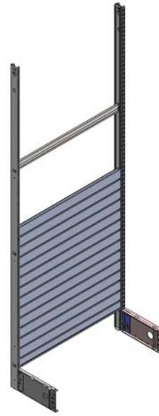
5 Install the next Slatwall Tie Bar. Same as step 3.
