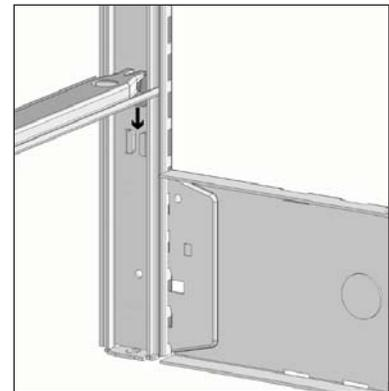
**2** Install the Cross Tie by sliding it into the bottom shear form(s) of the upright. You may need to tap directly above the tab with a rubber mallet to properly seat it. See illustrations above.
