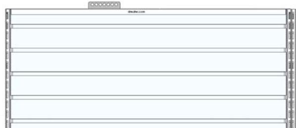
**8** Determine the location of the wall stud and mark with painters tape at the top of the gondola. Slide the Top Cap Anchor Bracket as shown above. A rubber mallet may be needed to slide the bracket to the approximate location of the wall stud.
