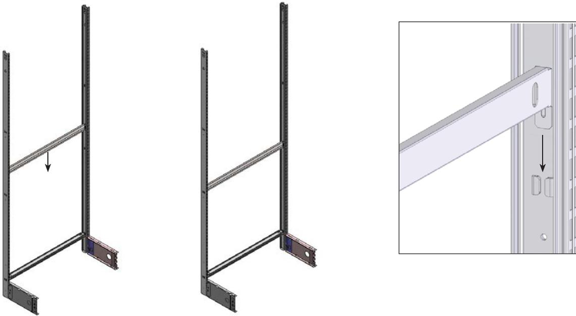
**3** Install the Slatwall Tie Bar into the shear form as shown. You may need to tap directly above the tab with a rubber mallet to properly seat it. See illustrations above.
