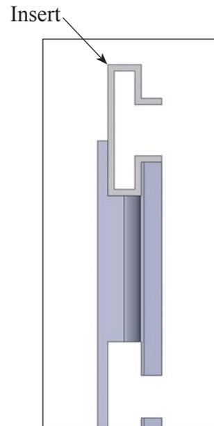
6 Place a piece of Slatwall insert in the top groove of the Bottom Slatwall. See figures above.
