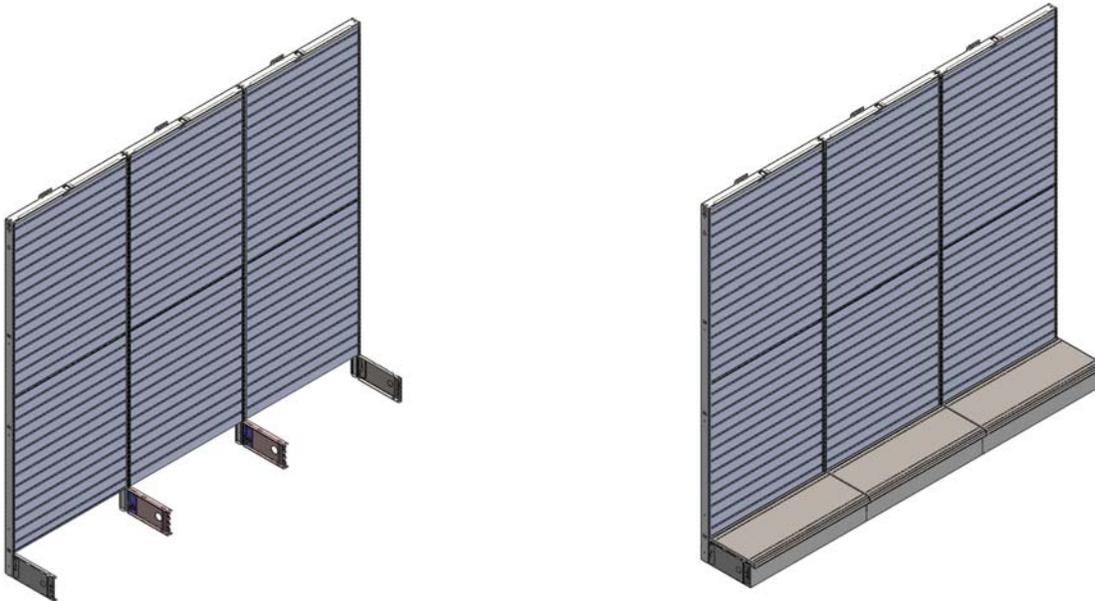
**12** Complete the rest of the run. Notice (2) End Standards and End Bottom Arms at the ends while the middle of the run contains Center Standards and Center Bottom Arms.
