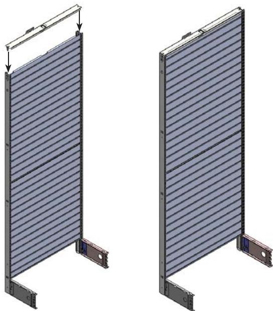
**9** Install the Top Cap into the the top shear form as shown. You may need to tap directly above the tab with a rubber mallet to properly seat it. See illustrations above. Secure the Top Cap Anchor to Stud.
