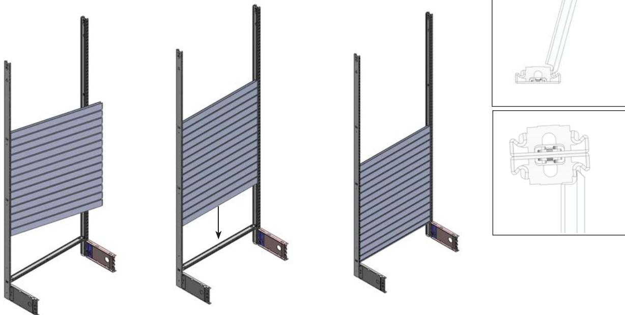
**4** The bottom and shorter piece of Slatwall will be installed as illustrated above. With the beveled edge facing outward, place the side of the slatwall into the groove of the upright. Next, simultaneously push the standard outward while twisting the other other standard so the slatwall pops in. Slide down.
