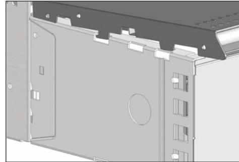
**11** Tip the Deck up slightly and slide it into the slots of the bottom arms. When properly installed, the deck should not tip forward when you push on the front of the deck.
