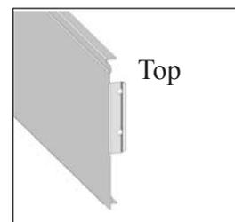
**10** Align the Kick Plate tabs with the fingers of the bottom arms. Tap kick plate with your hand or a mallet to seat the tabs securely into the fingers of the bottom arm. Repeat for Center bottom Arm.
